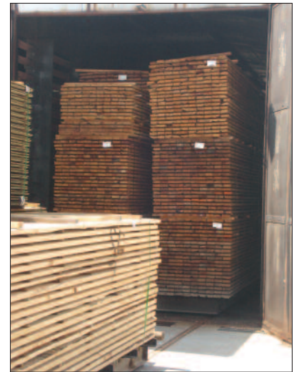
Properly drying and conditioning Southern Pine in a kiln helps reduce warping, splits and checks.
